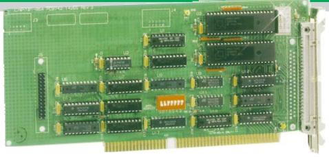
Low Voltage: 0.8 V max Low Current: -0.4 mA max High Voltage: 2.0 V min High Current: 20 µA max
